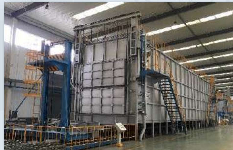
Heat Treatment Furnace 热处理炉
